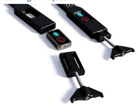
The smartbatten and system is designed to fit directly into the CT22 batten, and may accommodate other battens if required, or the sensor can be used as a standalone compression load sensor. The supplied case and tensioner assembly requires the batten to be shortened to accommodate the sensing unit. See the smartbatten System Dimensions drawing to remove the right amount from the batten.
